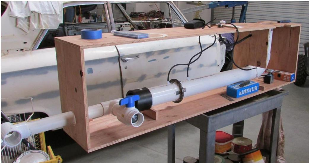
Figure 14, Completed Flow Bench
