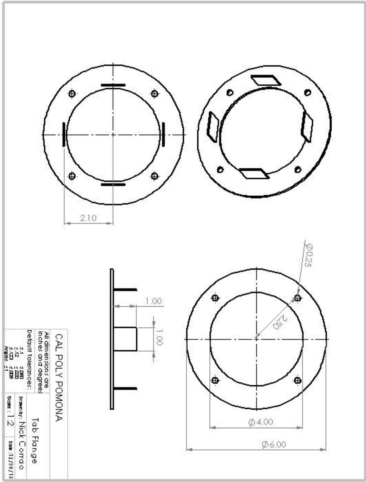
Figure 8, Tab Flange Drawing
