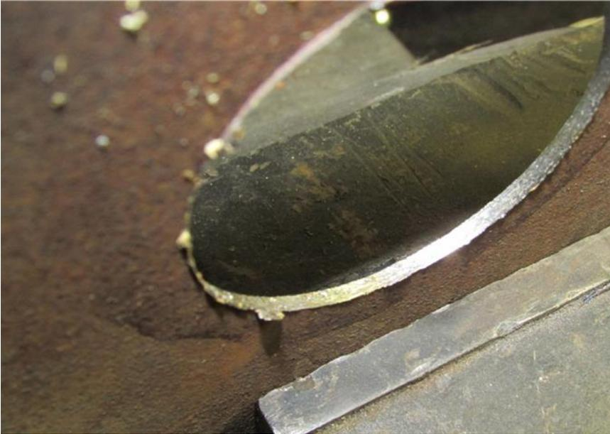
**Figure 9, Rough Cut Orifice Plate**
