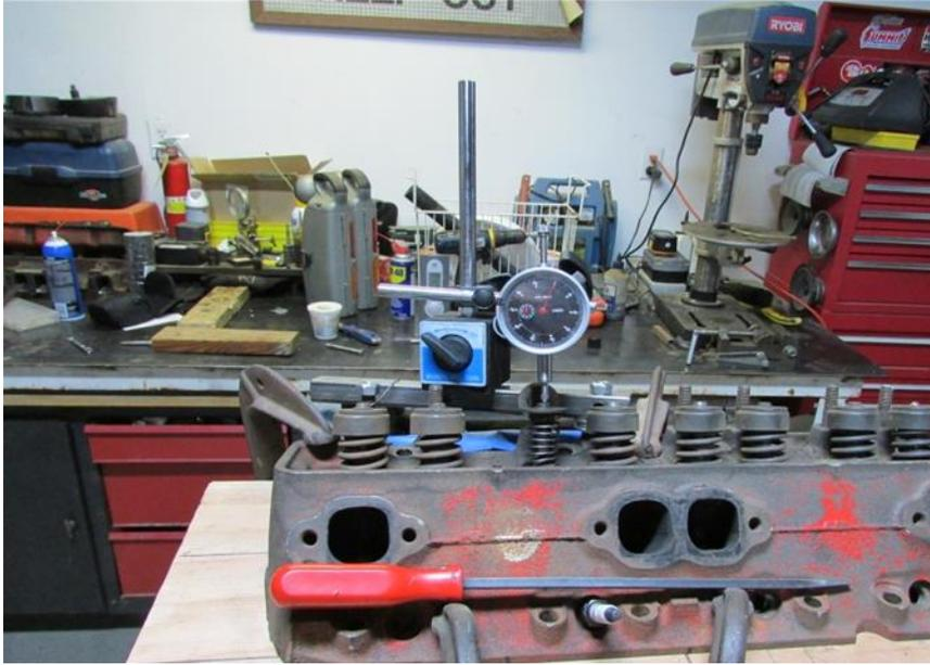
Figure 13, Head Set Up with Valve Depressing Apparatus
